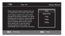
After selecting your TV's highest resolution, press the OK button, and the Wizard's aspect ratio screen will appear. NOTE: If you are unsure of your display's highest resolution, select "Auto" and BDS will select the optimal resolution for you.
